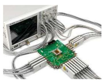
2- to 16-channel TDR/TDT/S-parameter measurement system.
