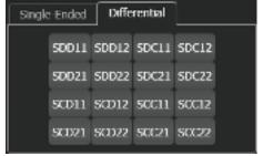
Select S-parameter measurements quickly and easily.
