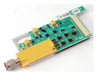
A high-speed step generator, sampler, and diode limiter are integrated into a proprietary microcircuit design housed in the remote head.
