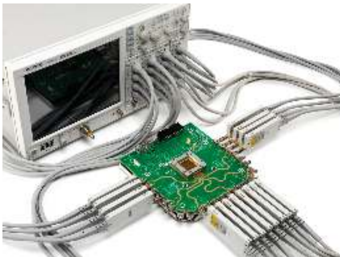
2- to 16-channel TDR/TDT/S-parameter measurement system.
