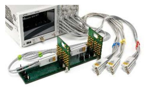
Perform efficient near-end crosstalk (NEXT) and far-end crosstalk (FEXT) measurements on differential designs that have up to four lanes.
