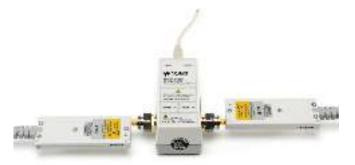
$\,$  N4694A DC-67 GHz electronic calibration (ECal) modules make TDR calibration and de-skew fast and easy.
